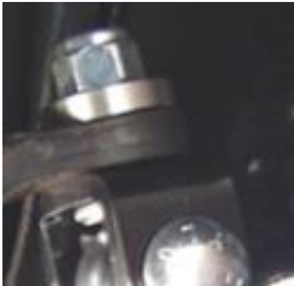
Billet Stainless Steel Washer Installed
