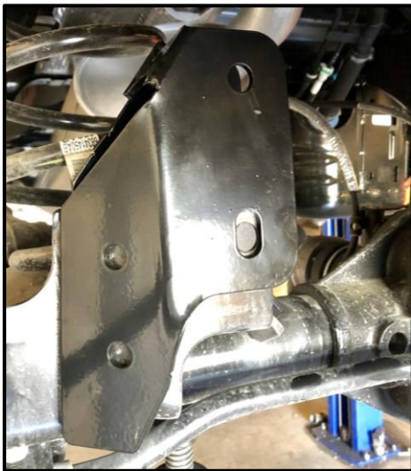
Driver Side Holes to Be Drilled
