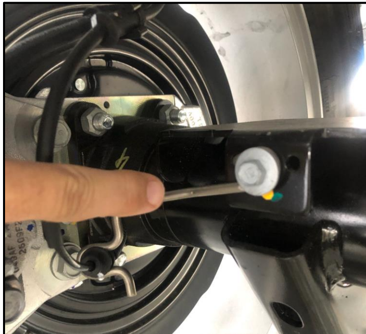
Brake Line Wire Form to be Removed
