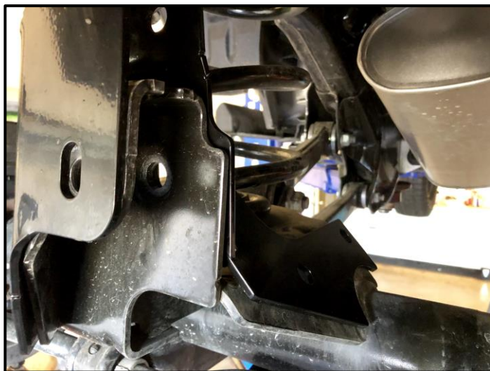
Pass. Side Holes to Be Drilled
