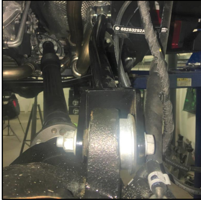
X Factor Driver Side Front Upper Arm Showing Proper Bend Orientation (Away from the frame) X Factor Pro: Is a straight double adjustable Aluminum arm (Not Shown)
