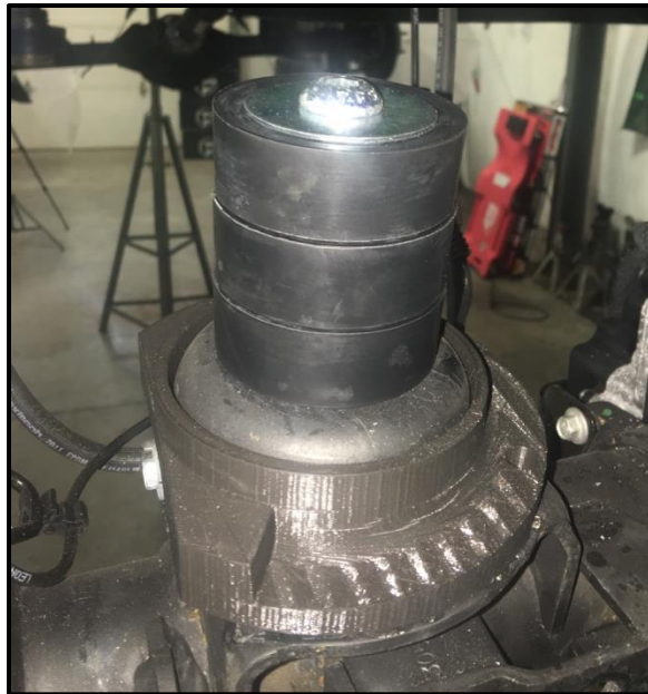
New Bottom Spring Seats Shown with Bump Stop Stack in Place
