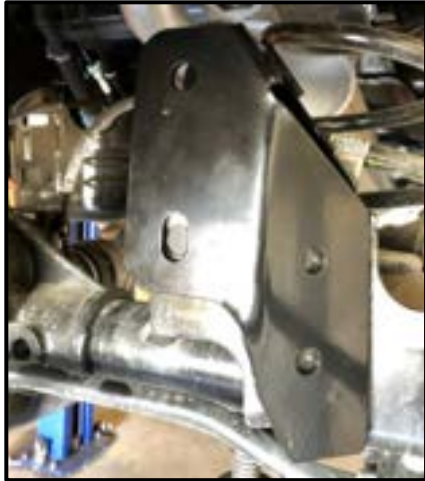
Driver Side Holes to Be Drilled
