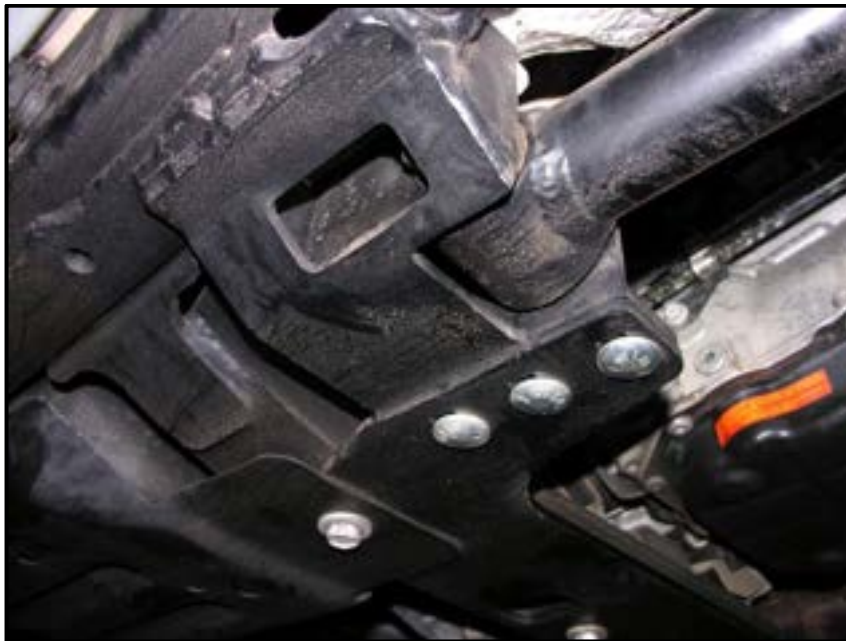
Finished long arm assembly (passenger side)
