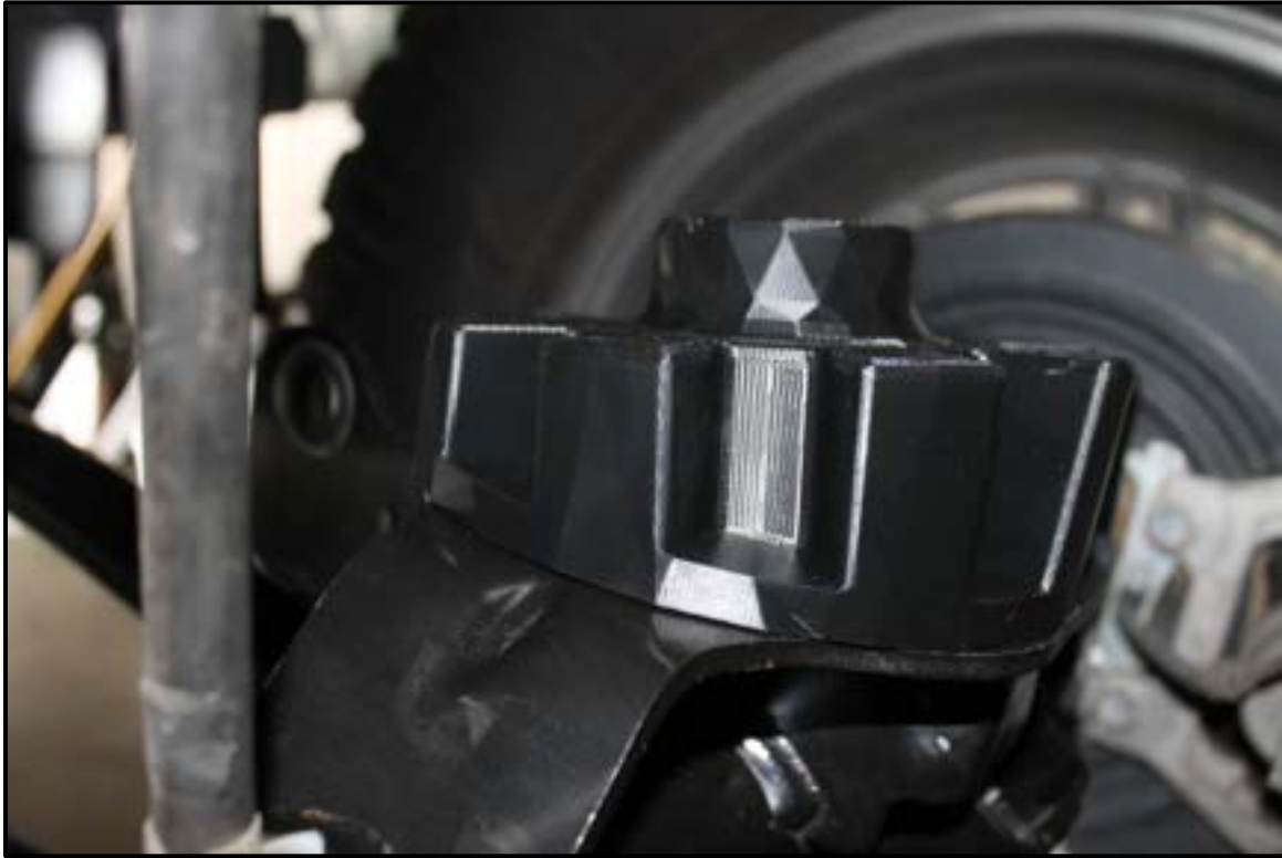
Pass. Side Rear Spring Seat Shown Installed
