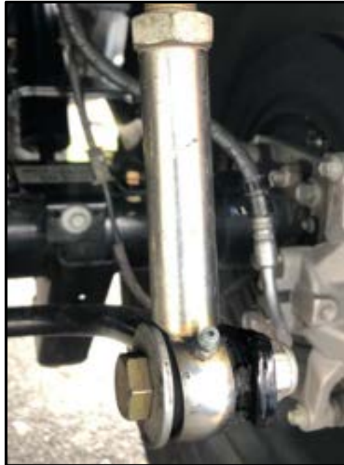
Rear Sway Bar Link Bottom Connection
