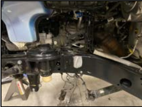
Passengers Side Bracket Removed
