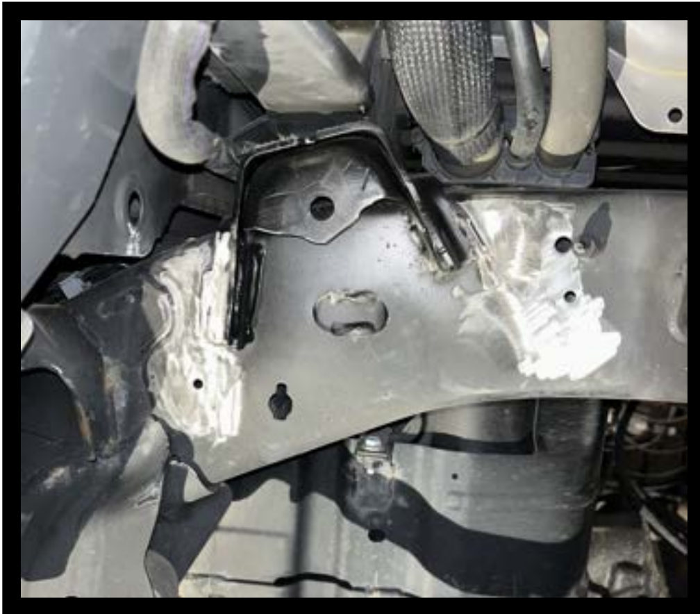
Rear OEM Shock Face Removed (Driver Side Shown)
