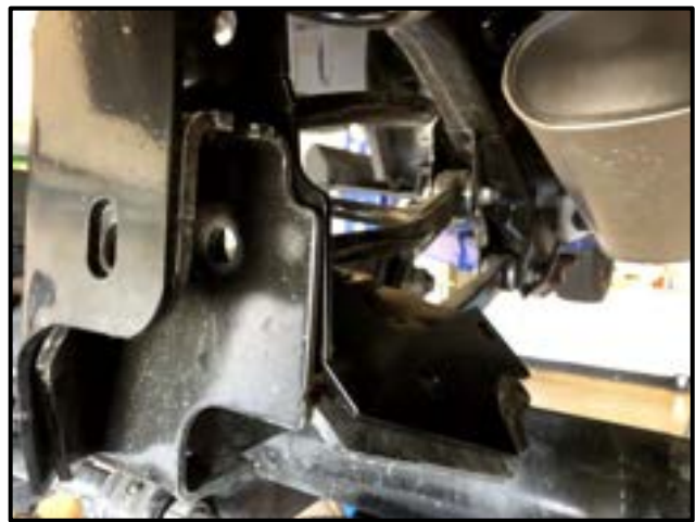
Pass. Side Holes to Be Drilled
