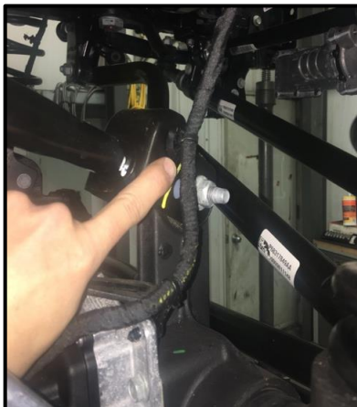
Remove Brake Lines from Arms
