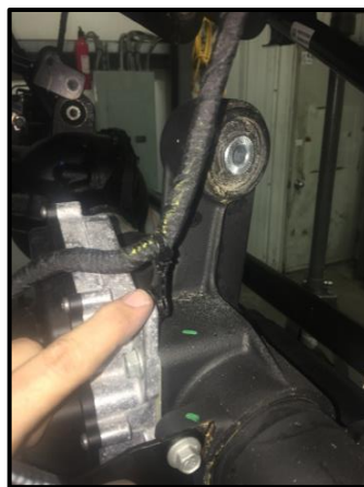
Remove Brake Lines from Arms
