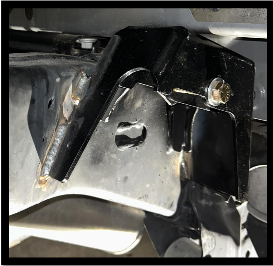
Top Shock Mount Welded in Place (Pass. Side Shown)
