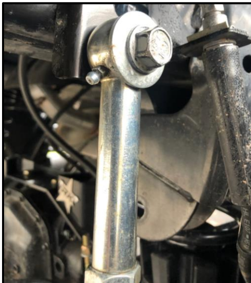
Rear Sway Bar Link Bottom Connection
