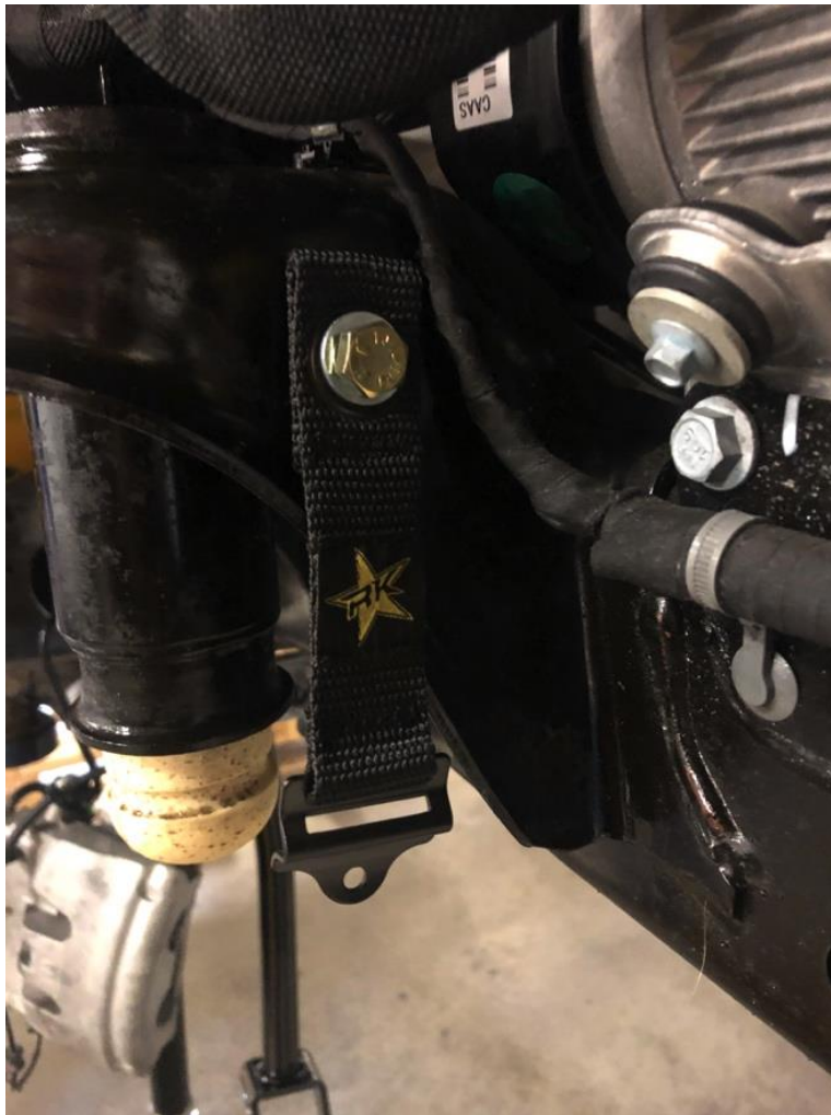
Sway bar strap retainer installed
