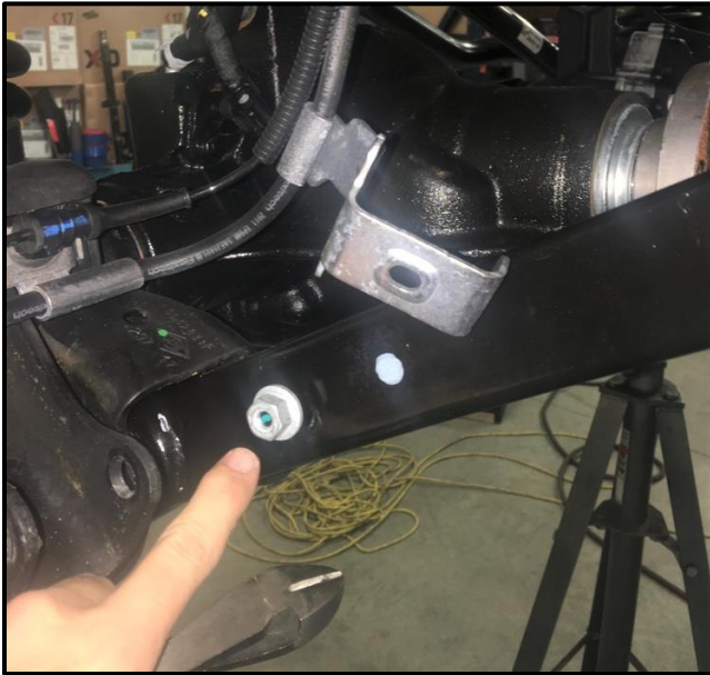
Remove Brake Lines from Arms
