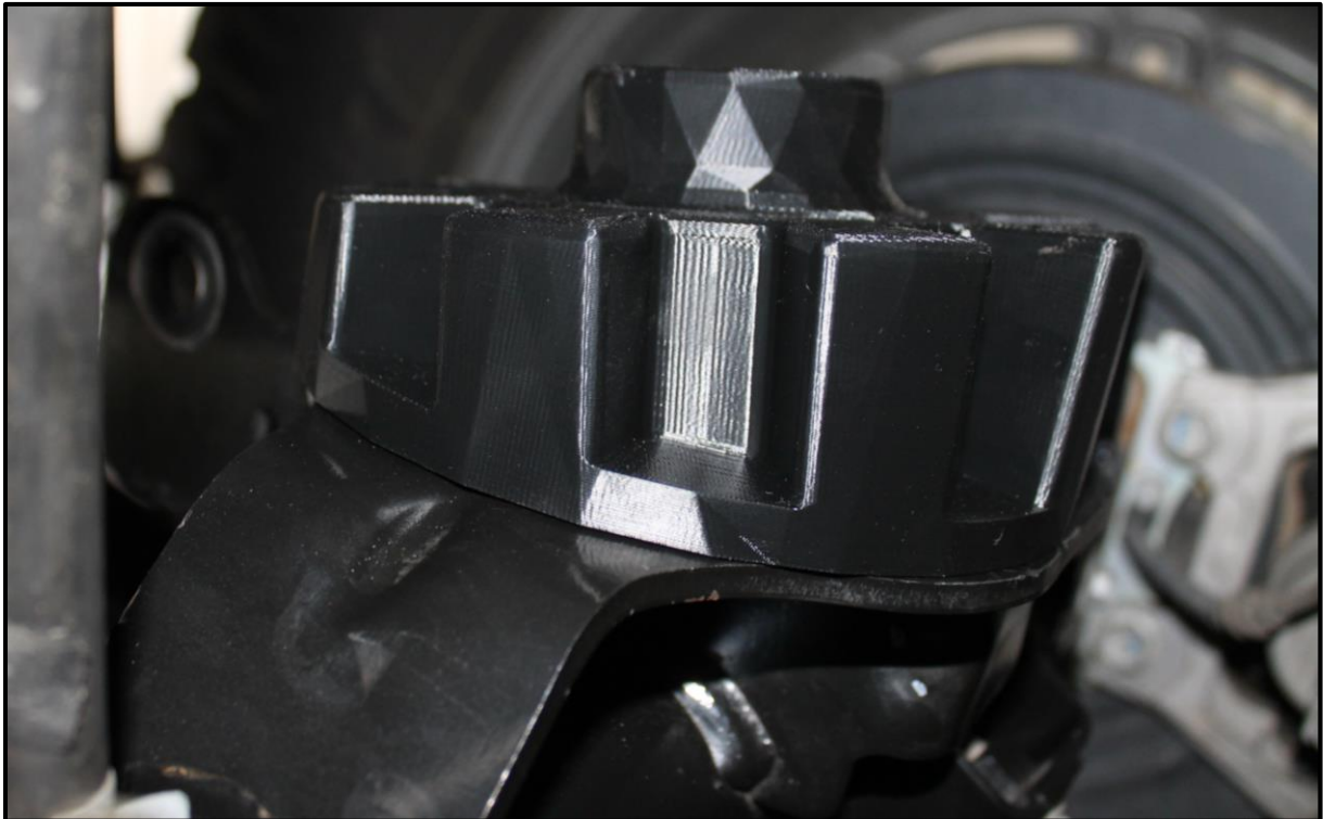
Pass. Side Rear Spring Seat Shown Installed
