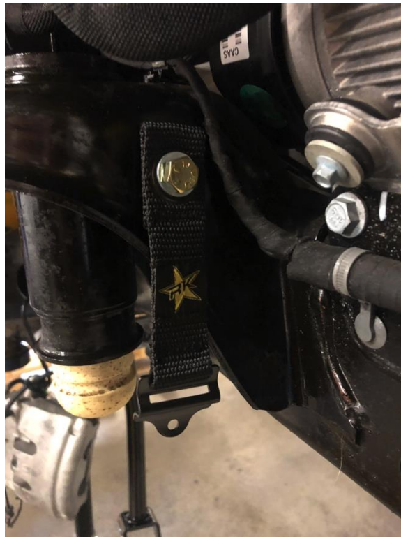
Sway bar strap retainer installed
