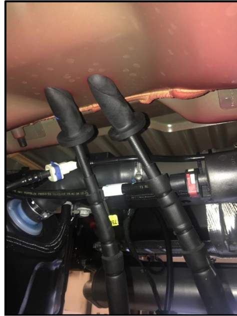
E Brake Cables routed ahead of the cross member
