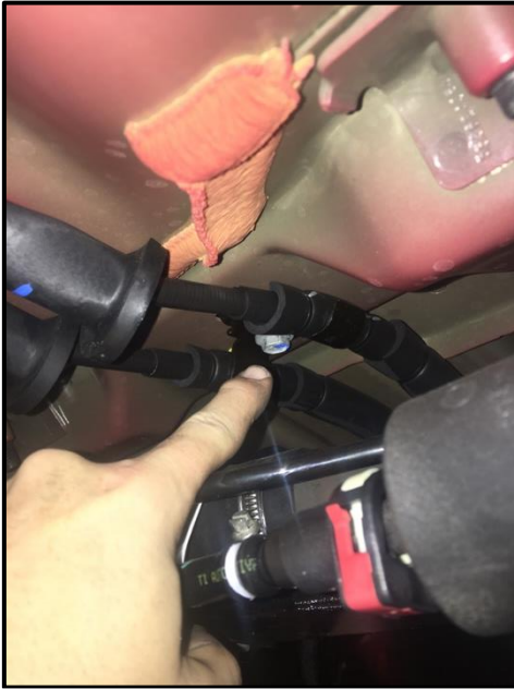
E Brake Cables routed ahead of the cross member
