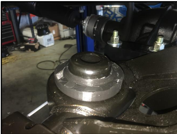
Driver Side Spring Seat Installed
