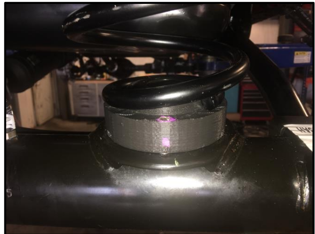
Pass. Side Spring Seat Installed with Coil
