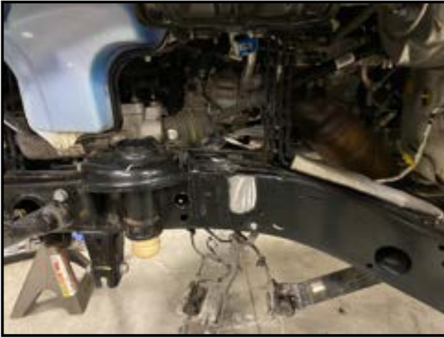
Passengers Side Bracket Removed
