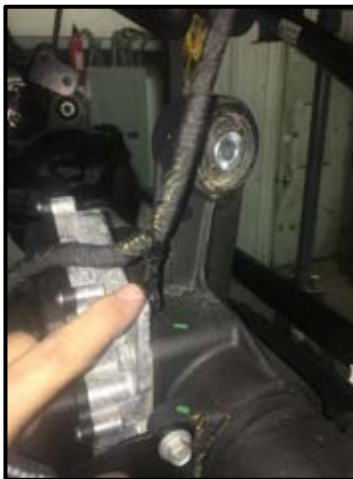
Remove the plastic clips holding the pass. disconnect motor cable from the upper arm and motor housing as shown
