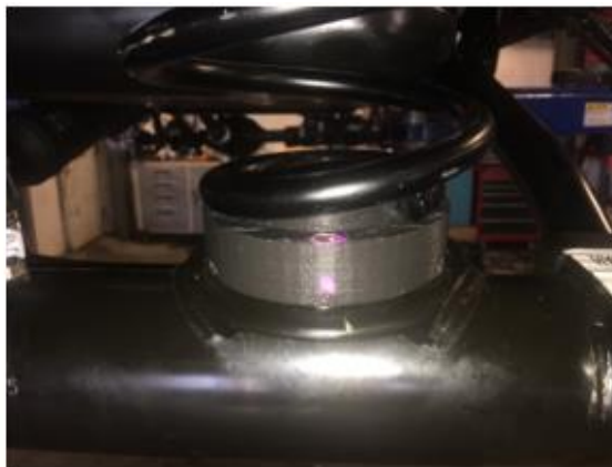
Pass. Side Spring Seat w/ Spring Installed
