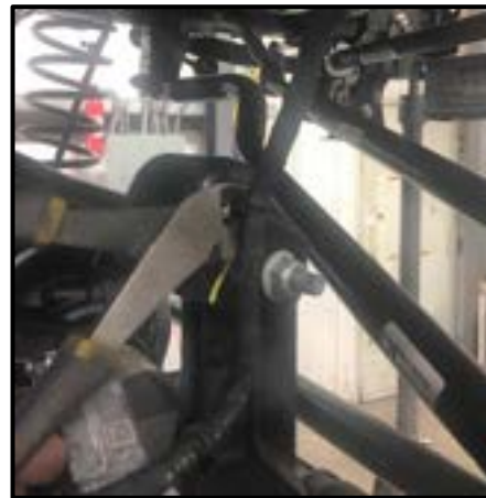
Remove the plastic clips holding the pass. disconnect motor cable from the upper arm and motor housing as shown
