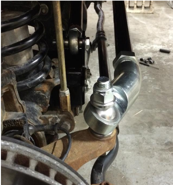
Passenger side knuckle connection
