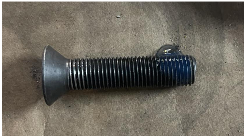
Blue Loctite applied to the 7/16 tooling bolt
