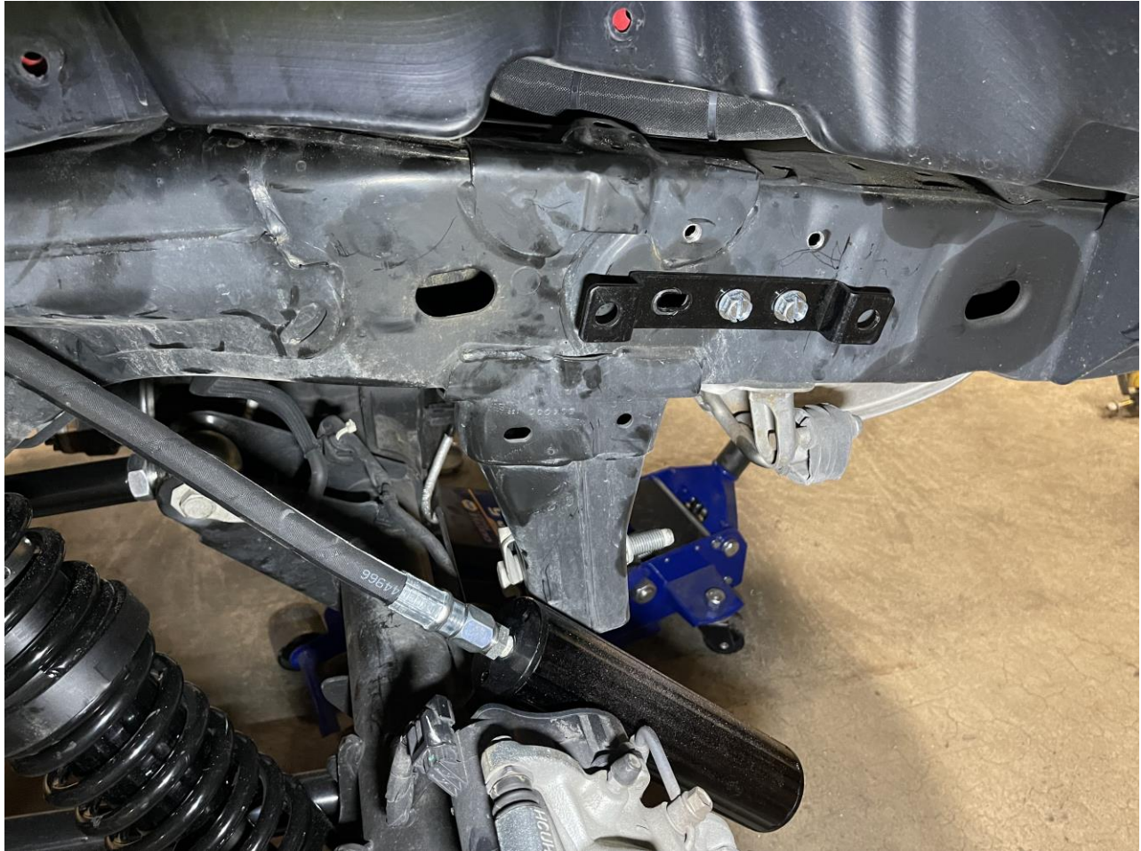
Rear Rassy Mount Installed
