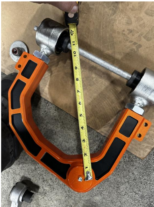
Driver Side Billet Upper A Arm Set to Match the OEM Dimensions
