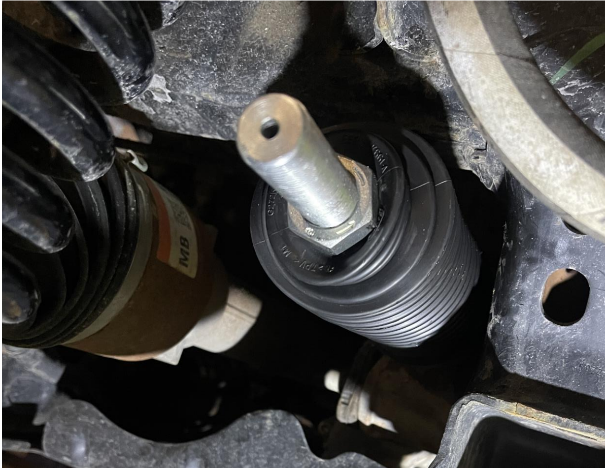
Boot and Jam Nut Installed
