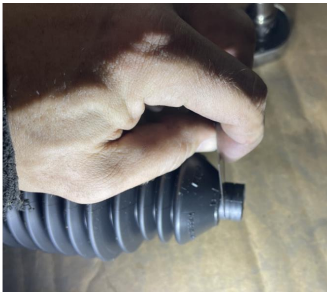
For Hoss 2.0 Trim the Small Lip of the Boot off as Shown above with a Razor Blade
