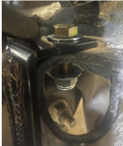
\frac{7}{16} Bolt, Washers and Nylok Nut
