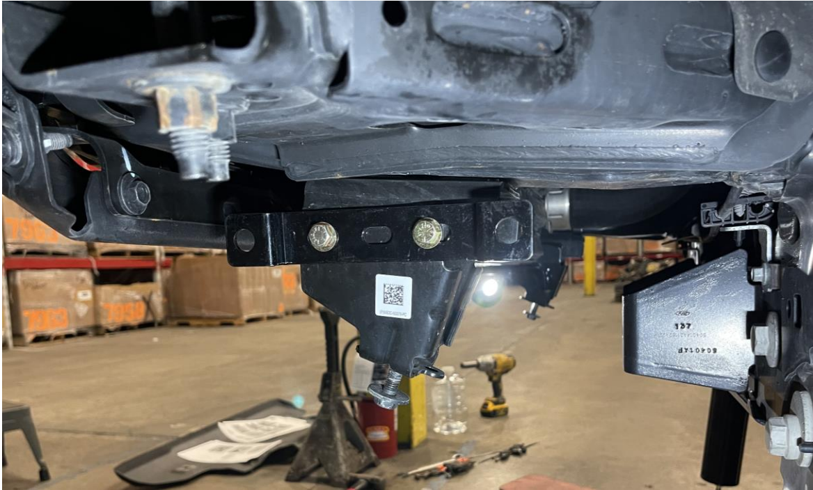
Rassy Bracket Installed (Driver Side Shown)
