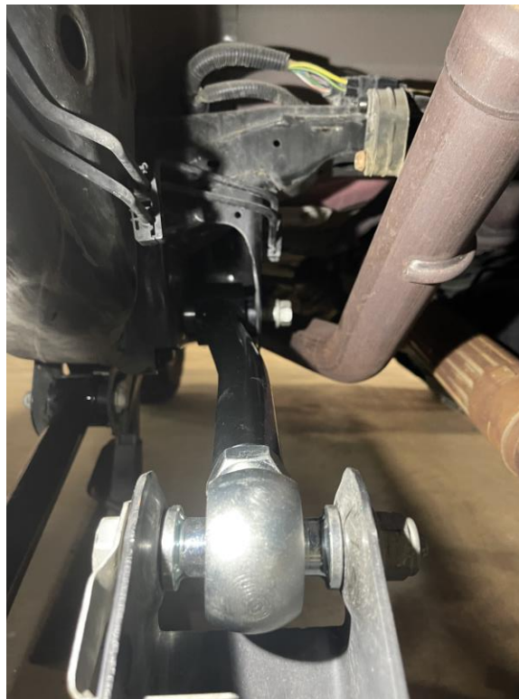
Driver Side Rear Upper Installed (Customer Opted for a Pro-X Krawler Joint vs. Adv. Series Joint No Longer Offered)
