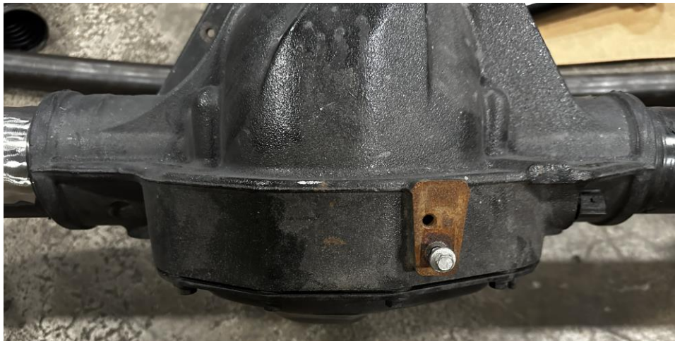
Rear Truss Alignment Hole(s)
