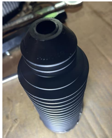
For Hoss 2.0 Trim the Small Lip of the Boot off as Shown above with a Razor Blade
