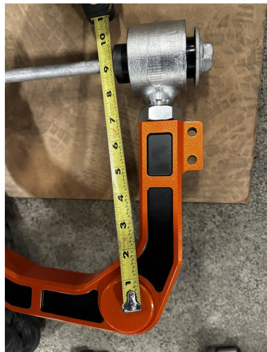
Driver Side Billet Upper A Arm Set to Match the OEM Dimensions
